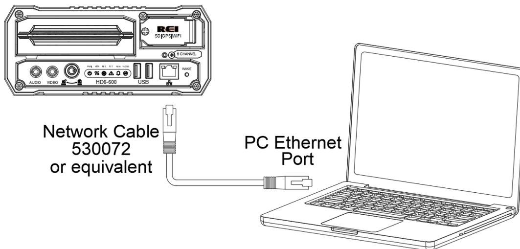
Figure 16: Connecting to the DVR with a Computer through the Ethernet Connection
