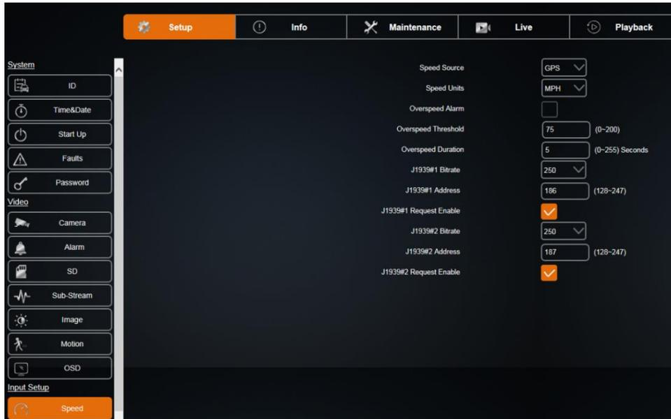
Figure 43: Speed Setup
