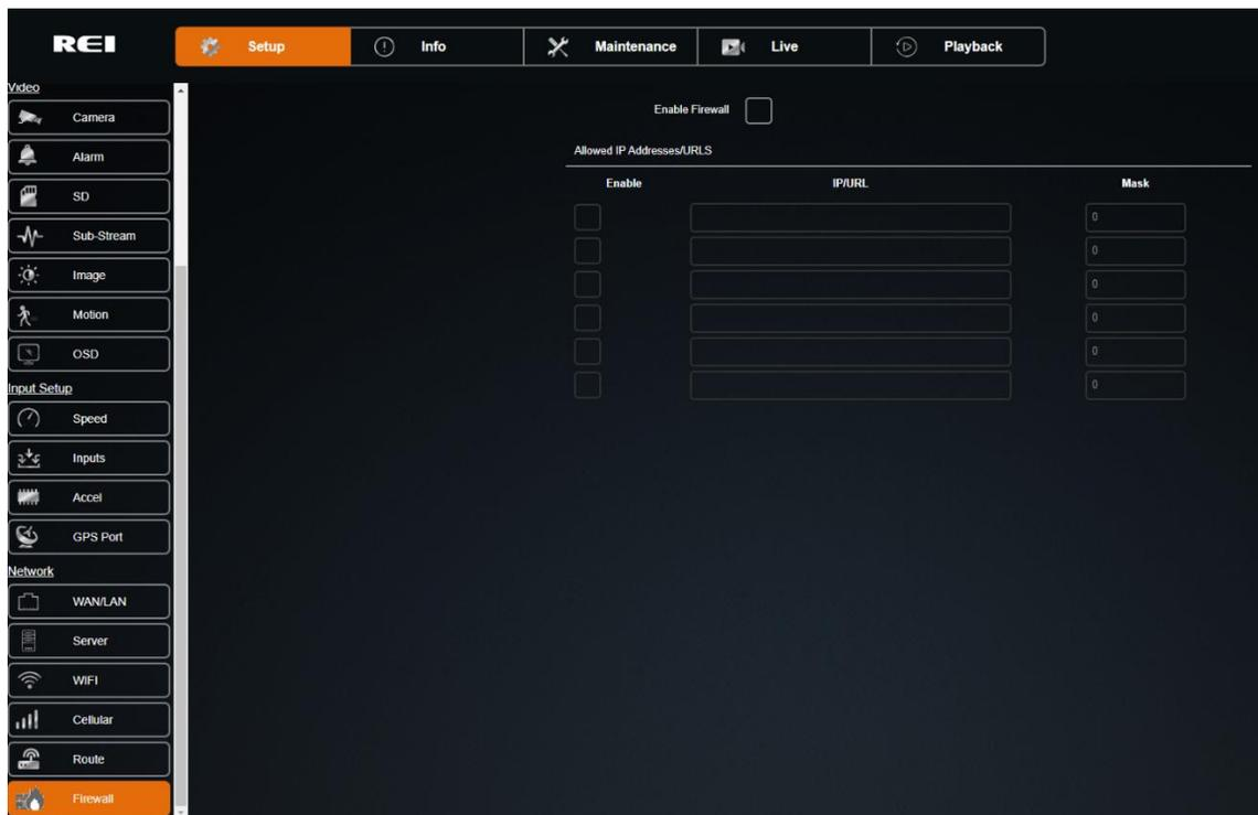
Figure 56: Firewall Setup
