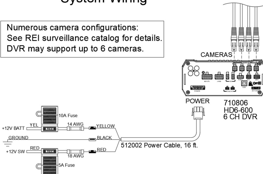
Figure 7: System Wiring - Power and Camera Cables
