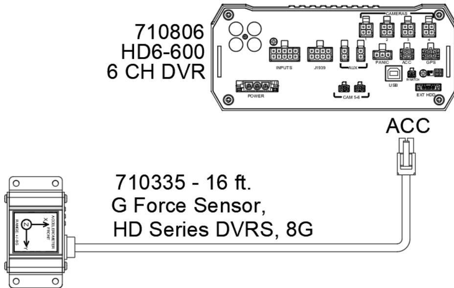
Figure 11: Accelerometer Module Harness Connection
