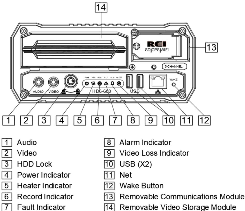
Figure 2: Front Panel Layout
