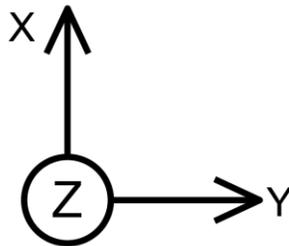
Figure 12: 3 Axis Inertia Sensor Directions
