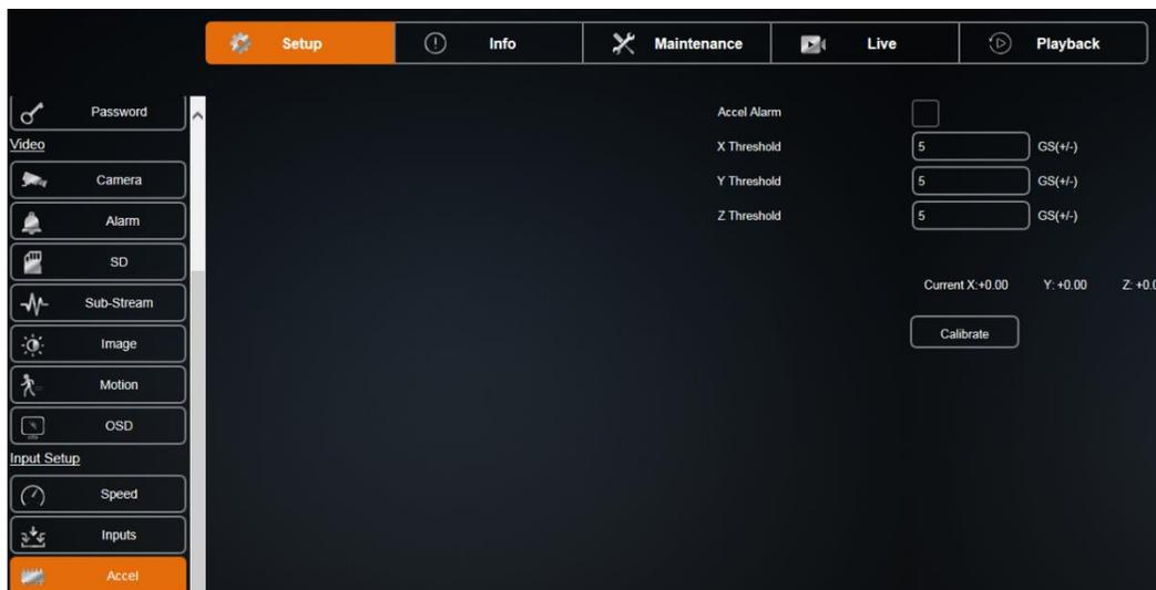
Figure 46: Accelerometer Setup
