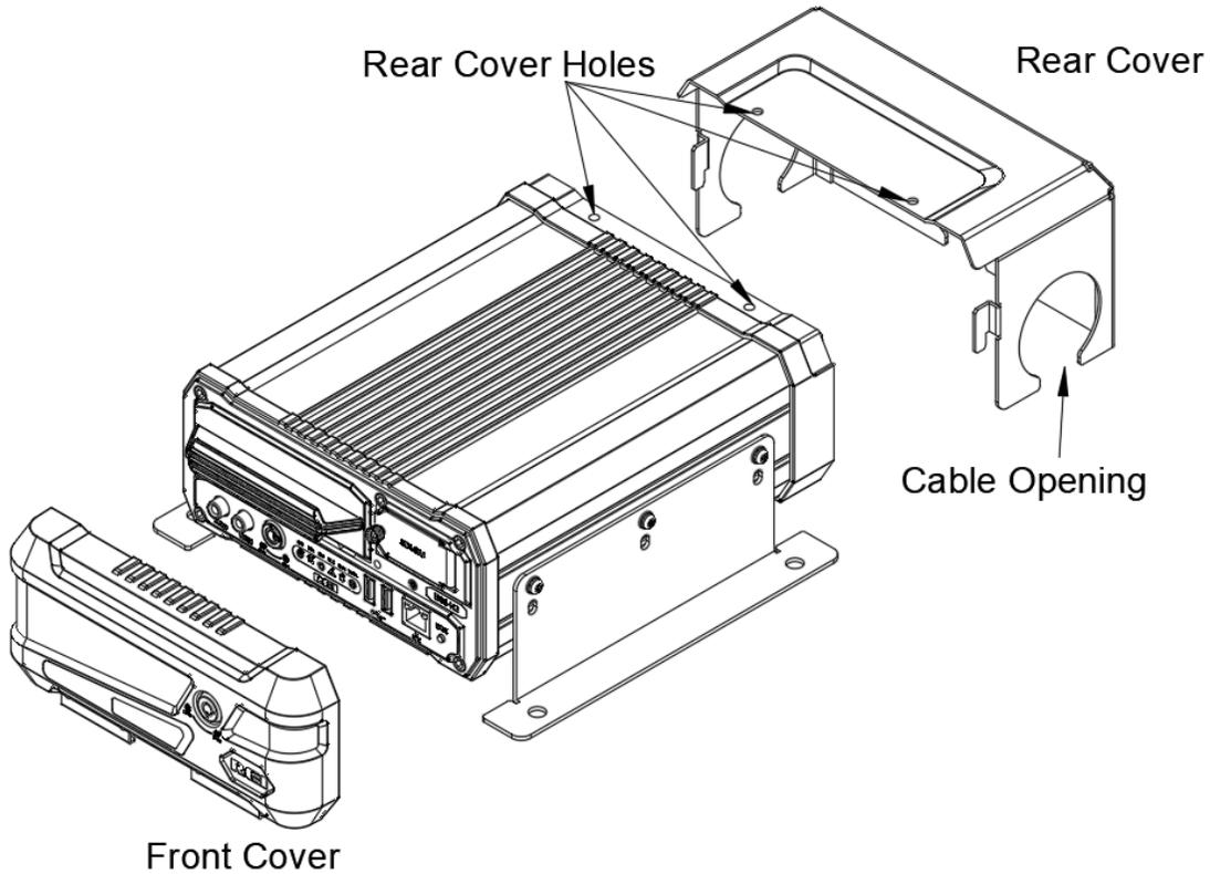
Figure 15: Security Cover Mounting
