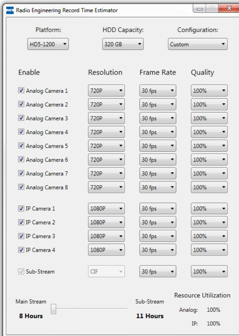
Figure 6: Estimator for HDD Record Times (HD5 shown)
