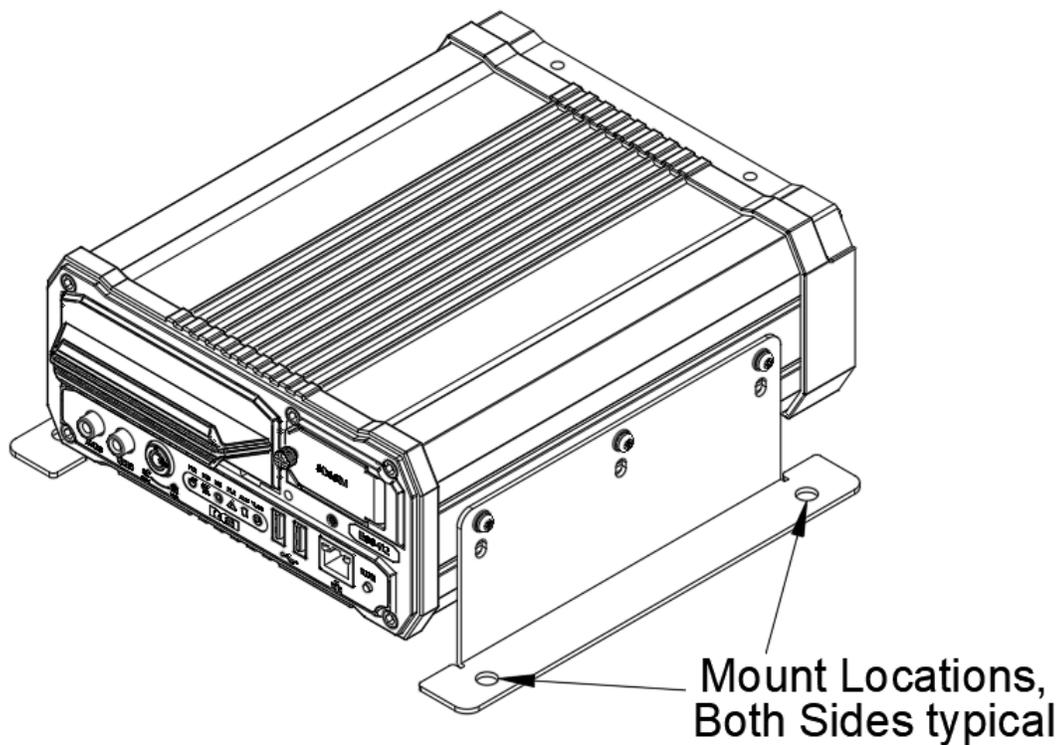
Figure 13: L Bracket Mounting
