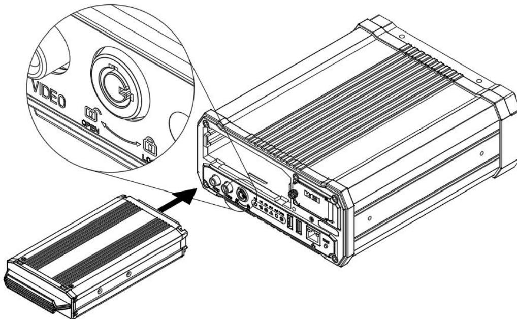
Figure 4: Removable Hard Drive Module
