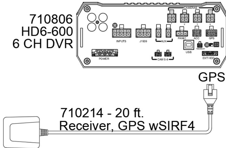
Figure 9: GPS Antenna Module Harness Connection
