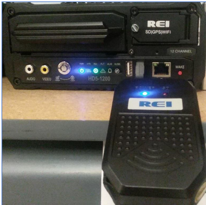
REI Toolkit Dongle connected to a DVR and operational
