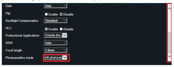
7. Left click on any tab on the left-hand side to save the settings. The IR sensor is now configured.
